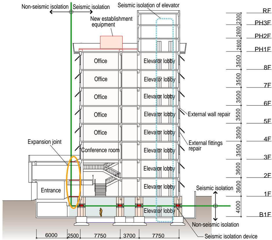
**Figure 7** Cross section
