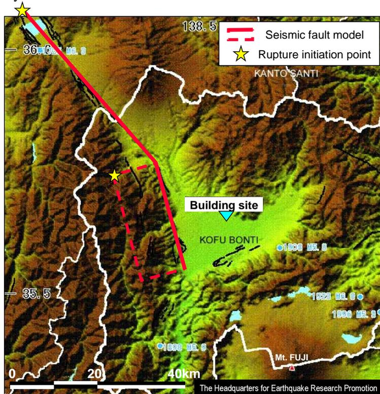
**Figure 2** Itoigawa-Shizuoka tectonic line seismic fault model
