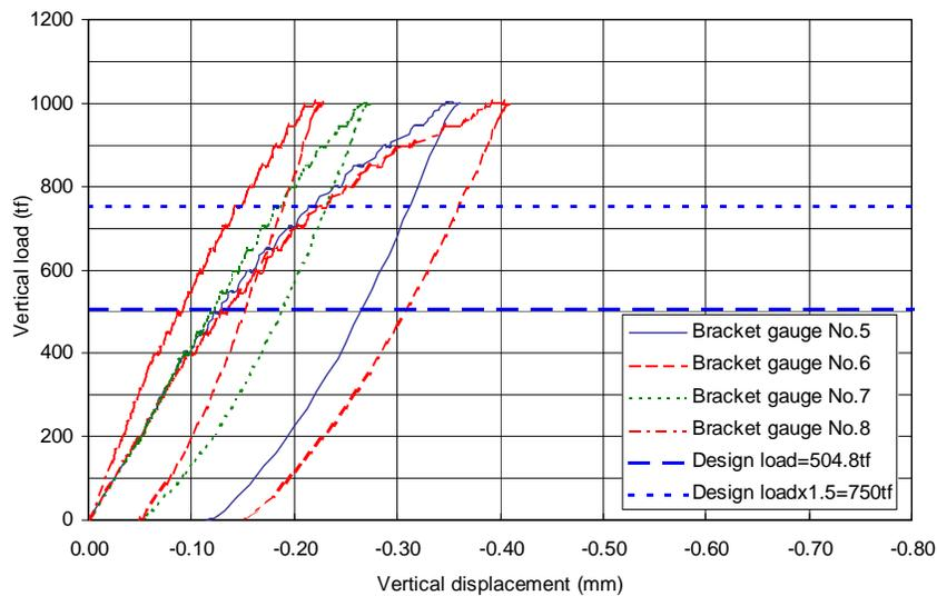
Figure 12 Experimental results (six-cable type)
