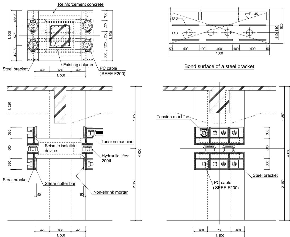
**Figure 8 Temporary supporting system (four-cable type)**
