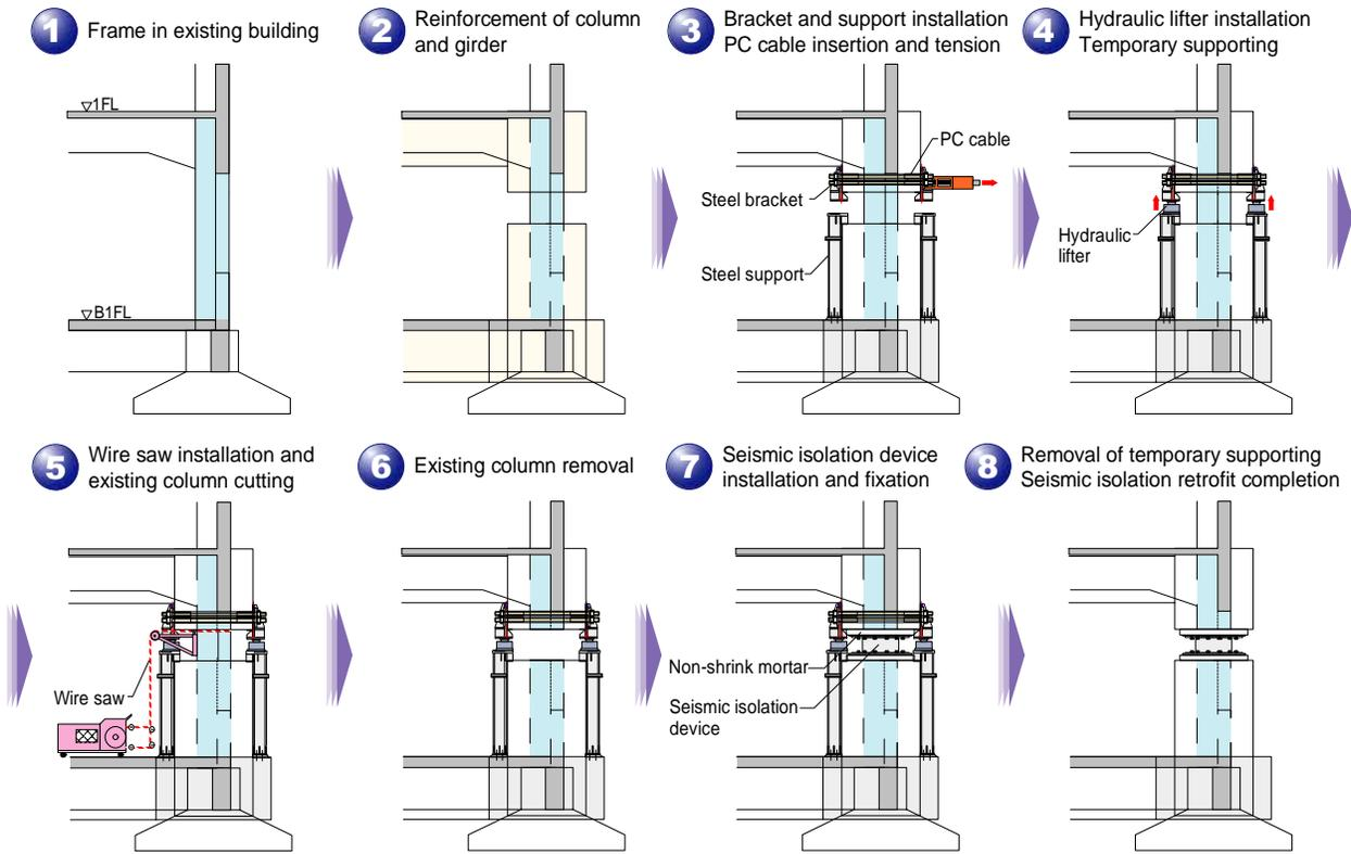
**Figure 14 Seismic isolation retrofit construction process**
