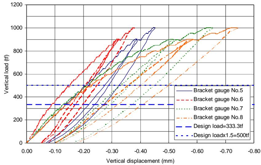
Figure 11 Experimental results (four-cable type)
