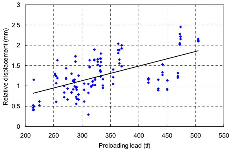
**Figure 15 Preloading load (equal to design reaction) - relative displacement relations**
