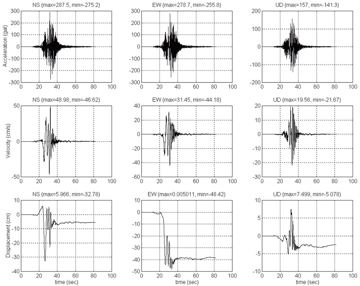
**Figure 5 Time history waveforms of acceleration, velocity and displacement**
