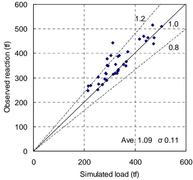
**Figure 18 Relation between simulated load and observed reaction**
