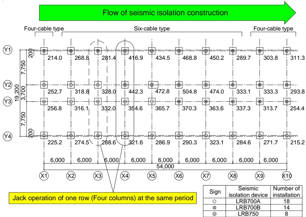
**Figure 13 Layout of seismic isolation devices with design reaction force of column (tf)**
