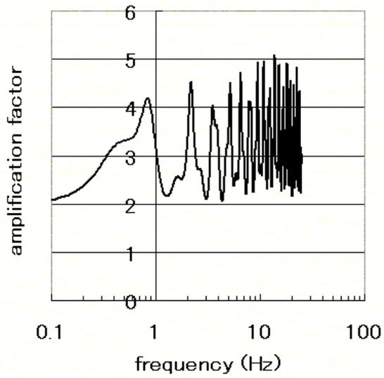
**Figure 3 S-wave amplification**
