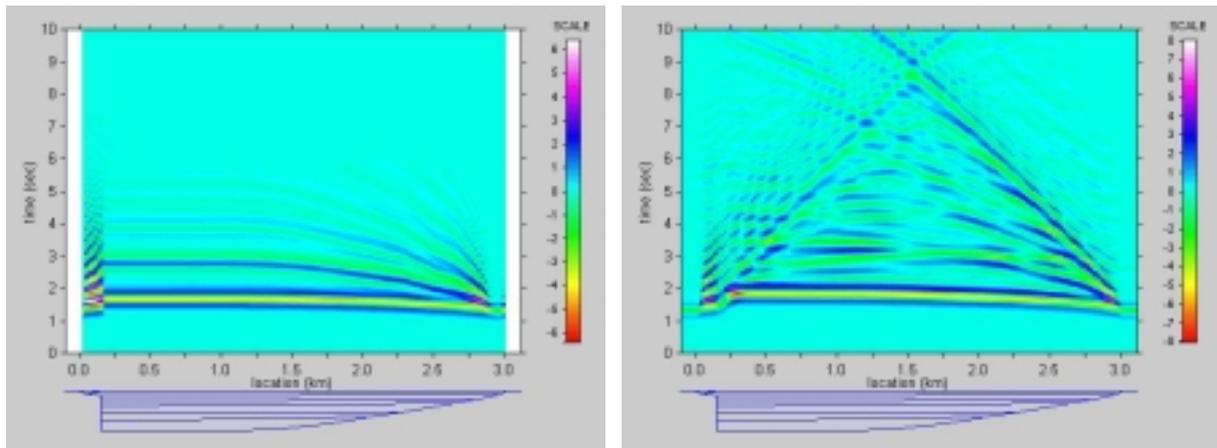
**Figure 3.** (a) 1D and (b) 2D synthetic velocity across a model of Lower Hut, NZ; vertically incident SH-wave with a Ricker pulse excitation with central frequency of 2 Hz (Adams et al, 1999; Adams, personal comm. 1999).
