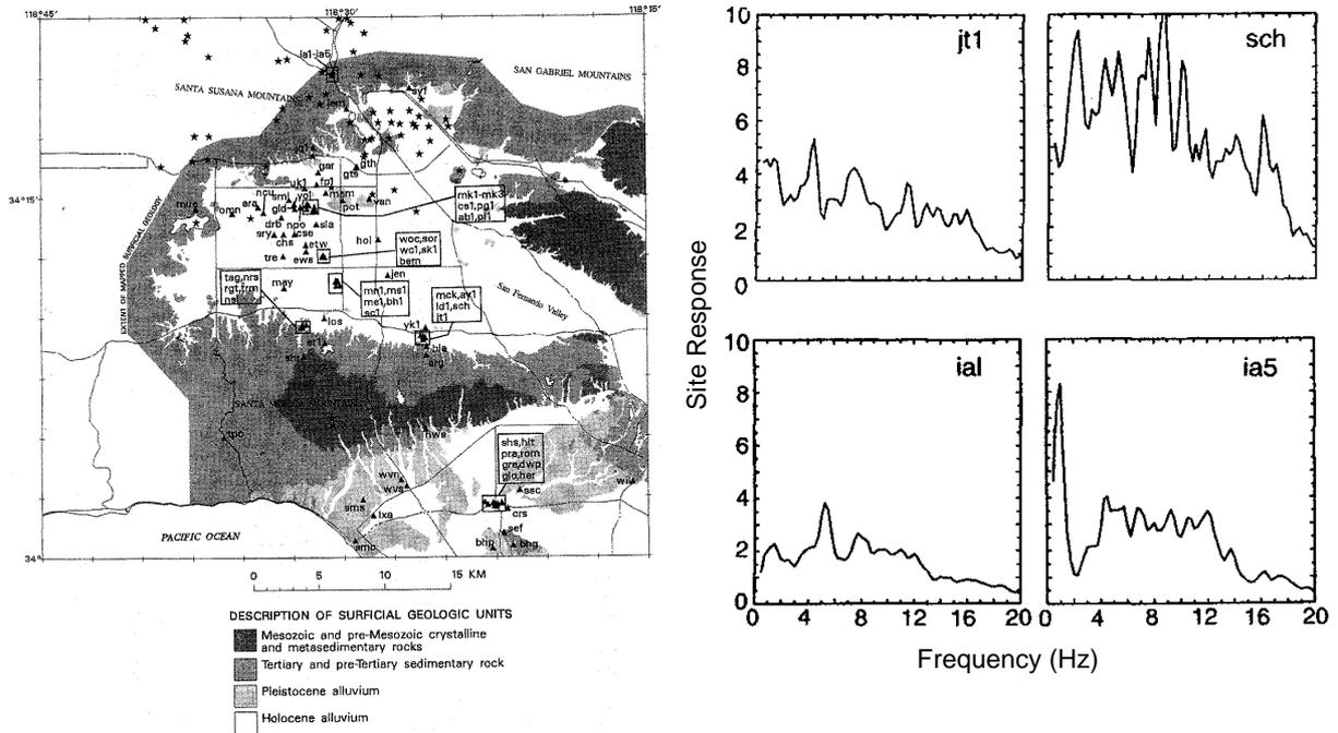
**Figure 8. (a) Location of sites in SFV instrumented for studying spatial variation of ground motion of 1994 Northridge earthq. aftershock; (b) spectral ratios at indicated locations derived from recorded seismograms (Hartzell et al, 1996).**
