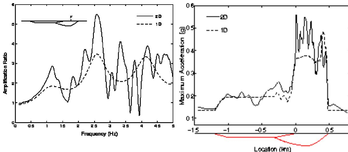
Figure 2. (a) 1D and 2D amplification ratios at site F (see insert) due to steady-state harmonic vertically incident SH-wave; (b) Maximum free surface 1D and 2D synthetic accelerations across a valley in Kirovakan during Spitak earthquake. Bielak et al (1999).
