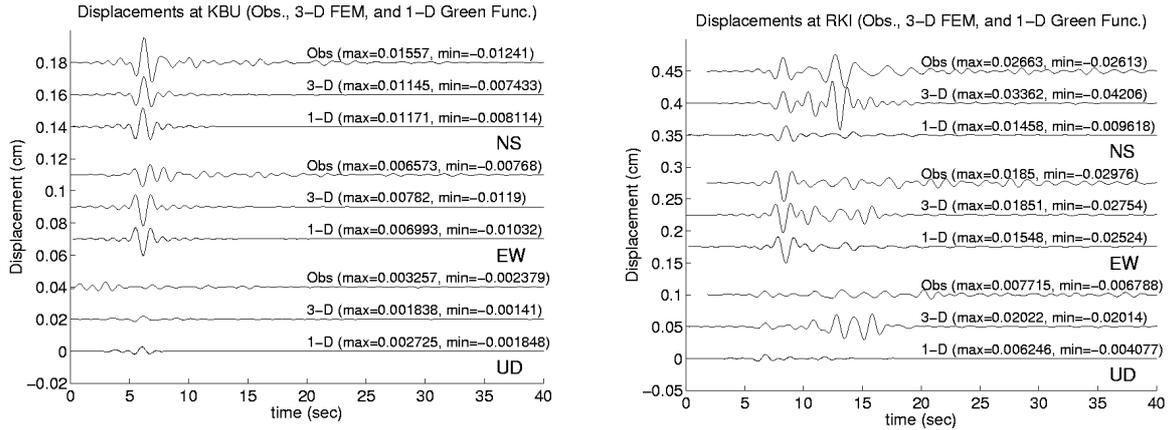
**Figure 7. (a) Band-passed displacements (0.9-5.0 s) observed and simulated for a 1995 Kobe earthq. aftershock at sites KBU and RKI (see Fig. 10a) (Hisada et al, 1998).**
